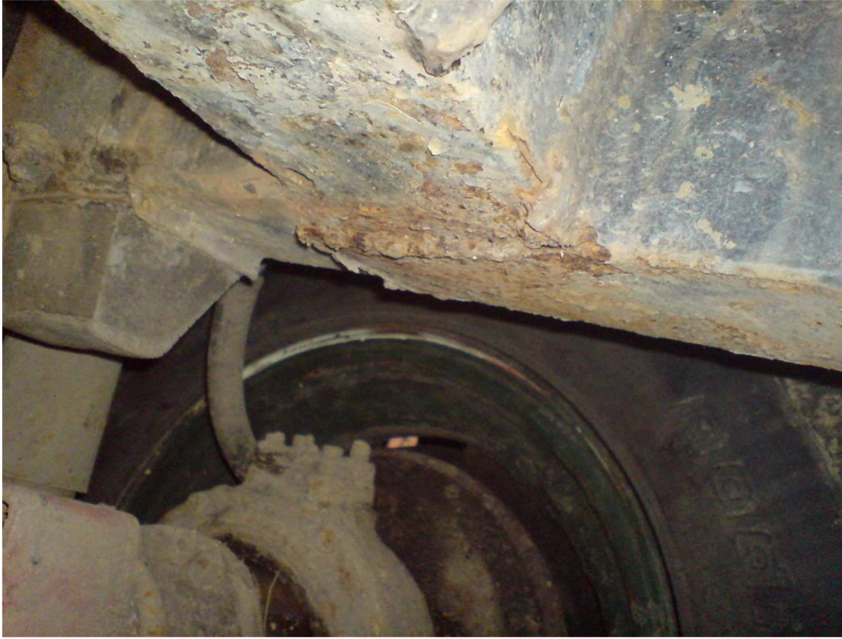
Just one example of an outrigger...the small holes were the start of it...it was shockingly thin....in the end I think every single outrigger was replaced:
